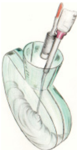
Fig. 4: Overflow protection of casts, for example for plastic lenses for glasses
