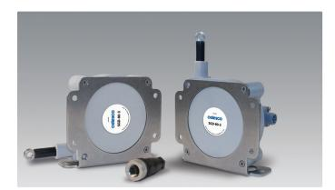
Suited for IP67 (wet) environments, the SGD provides a userselectable 4-20mA or 0-10VDC absolute linear position signal over an 80-inch or 120-inch full stroke range option. Signal selection is simply made by connecting the appropriate pins on the included connector or selecting the proper wires in the optional cordset.
