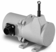
The PT8101, using a high cycle plastic-hybrid potentiometer, operates with any basic panel meter or programmable controller in factories and harsh environments requiring linear position measurements in ranges up to 60".
